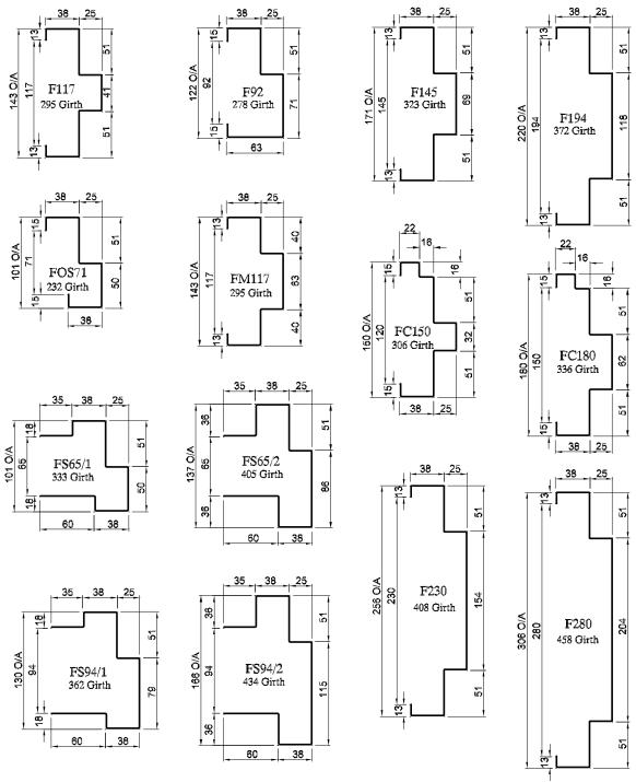
**Note:** When installed with appropriate door leaf, frames are fire rated up to 4 hours in masonry walls, and 2 hours in dry wall. Custom frame profiles available on request. Frames are typically 1.2-1.6 zincanneal unless otherwise requested.
